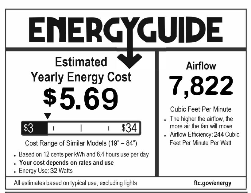
Airflow Shown Is a Weighted Average of High and Low Cubic Feet per Minute Based on Close to Ceiling
